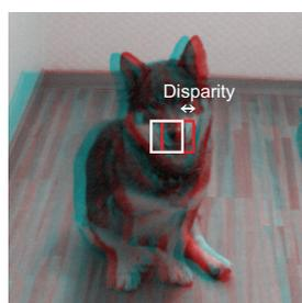
Fig. 7 Disparities between standard and reference images. Distance to the object is calculated from disparities.
