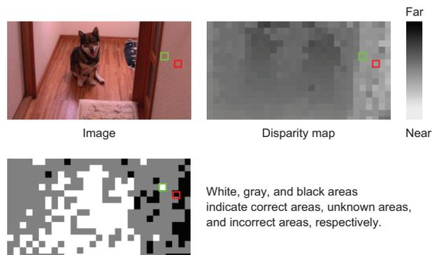
Fig. 13 Reliability of disparity map. Incorrectly measured distance can be corrected using more reliable distance of the neighborhood region with a similar color in the image.
